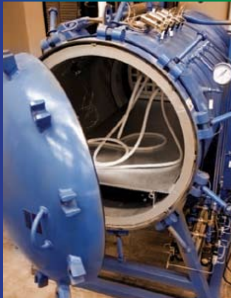
Trident Technical College's Aeronautical Training Center includes an autoclave to prepare students for working with composite materials.
